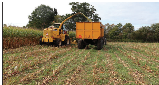
Figure 26. Corn silage being harvested with a self-propelled harvester. Photo: Shane Wood, Perennia.
