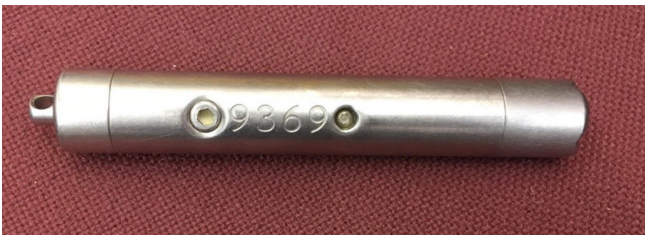
Data logger used to record rumen pH
