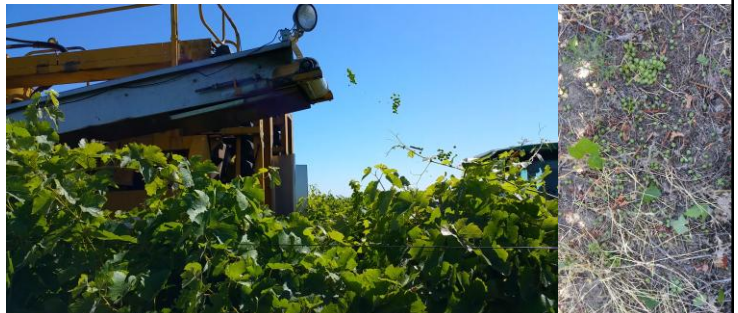
Ground speed 2.6 km/hr, shaking 425 rpm → Berry thinning
