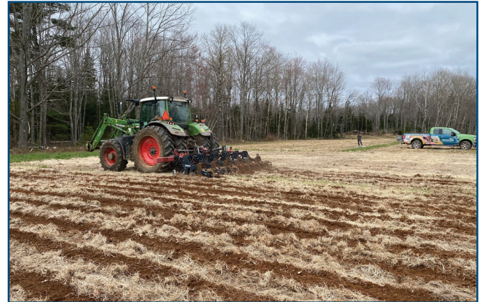
Figure 3. Strip tillage, where only the planting rows are tilled while the soil between rows remains undisturbed.
