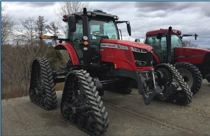
Figure 1. Tractor wheelbase is widened to approximately 11 feet, allowing four potato rows to be planted between the wheel tracks as part of a Controlled Traffic Farming (CTF) system. Photo Credit: Leigh Hunter, McCain Farm of the Future.
