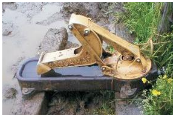
Figure 3.13 It is preferable to place a pad underneath the nose pump to avoid a mucky drinking area
