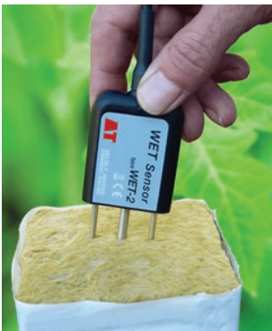
Figure 4. An example of a WET sensor. Having a mobile sensor can be helpful throughout the facility to account for microclimates that exist within the space. These devices can also help classifying moisture across a single pot/bag to see how that profile changes within a fairly restricted volume. Photo from Delta-T Devices ( https://delta-t.co.uk/product/wet-2-horticulture/ )
