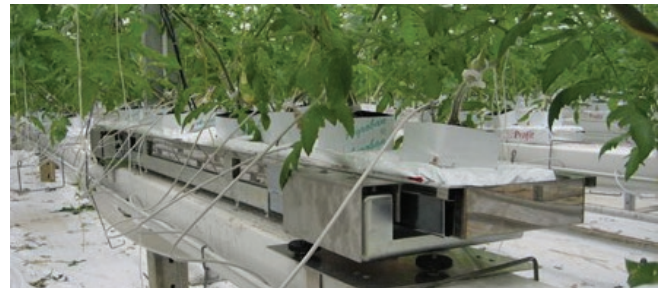
Figure 5. An example of a weigh station used for monitoring irrigation. When the slab is fully saturated with water, the higher weights will prompt the system to hold off on delivering additional water. As the slab dries out and the weight decreases, the scale will send information to the irrigation computer to deliver more water once a target weight has been hit. Photo from Agrofim ( https://www.agrofim.pl/en/19-oferta/szklarnie/158-root-optimizer )
