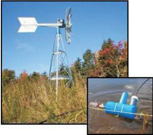
Figure 3.13 A 12-foot windmill driving a water pump with compressed air.
