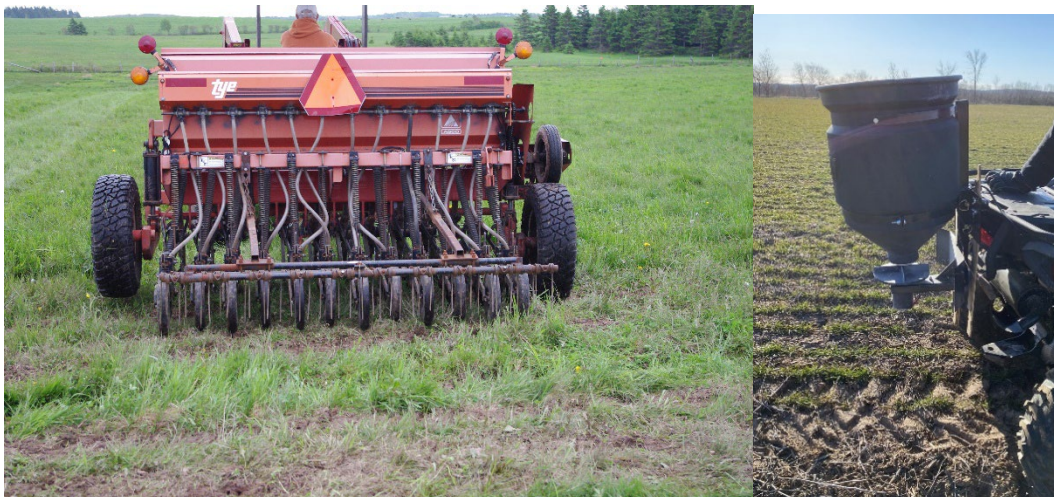
Figure 5.1 Different types of seeders. No-till seeder. Broadcast seeder mounted to an ATV.
