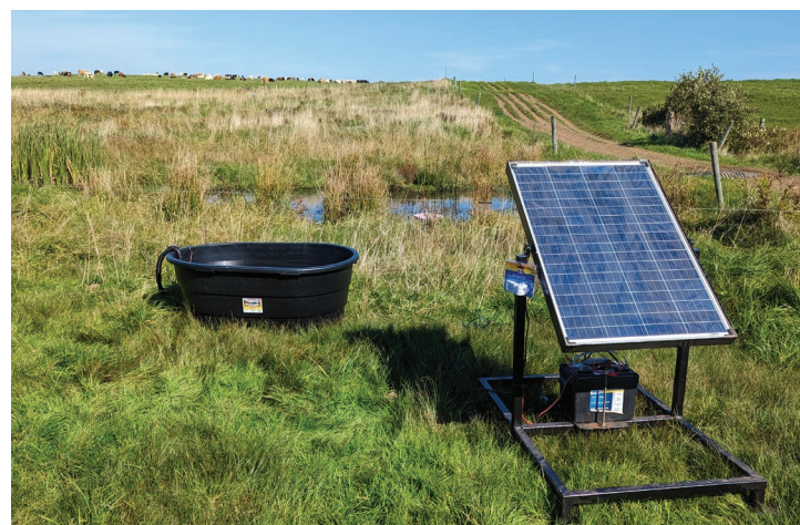
A DIY solar watering system moving water from a nearby stream into a tub. Keeping cattle out of watercourses protects riparian and animal health.
