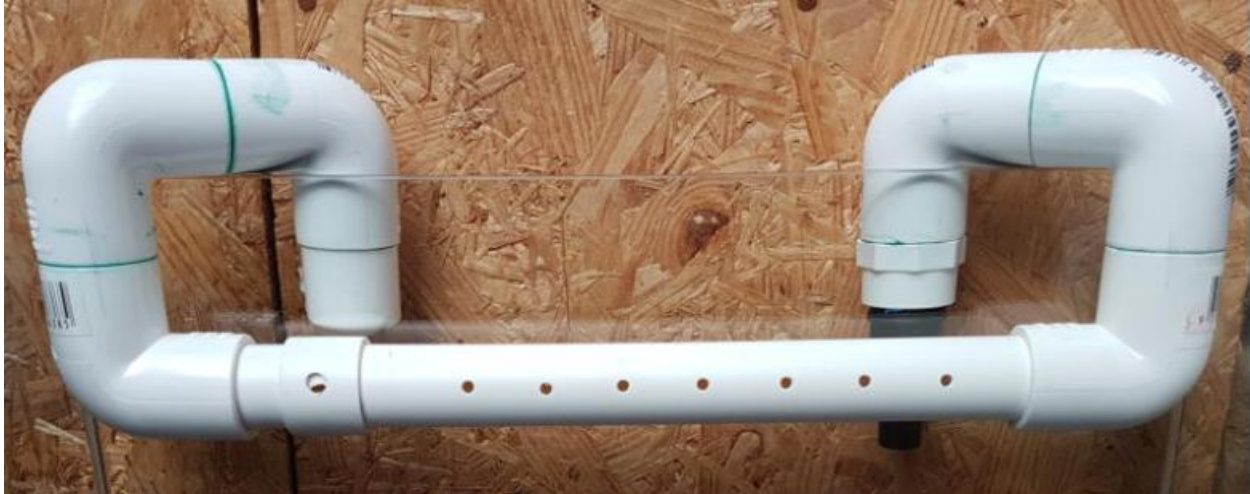
Figure 2. Schematic of a typical spray bar (Source: J Nickerson)
