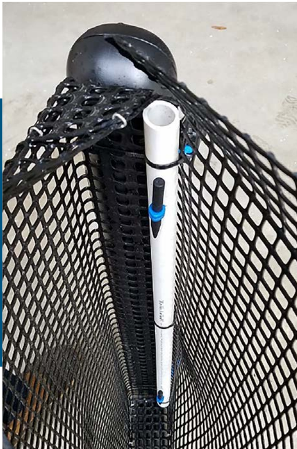
FIGURE 2. Use of a PVC pipe bar to reinforce bag and reduce friction where clips attach as one example of a method to reduce chafing. Photo courtesy of Outlaw Oyster Company
