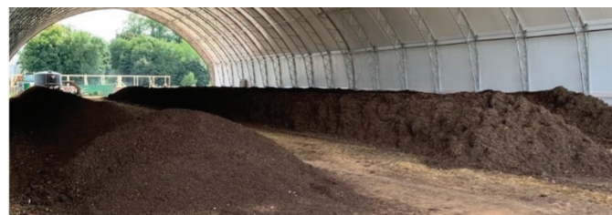
Figure 2: Windrow composting system
